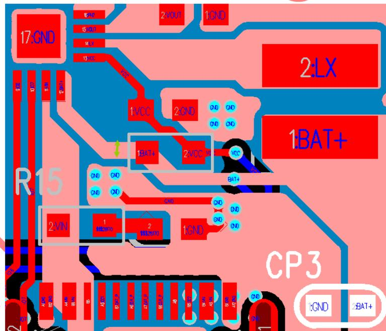
5. LX PIN is the connection PIN between the internal boost circuit and the inductance. There is a high-frequency switch signal on the LX wiring, so the wiring should be as short and straight as possible:
