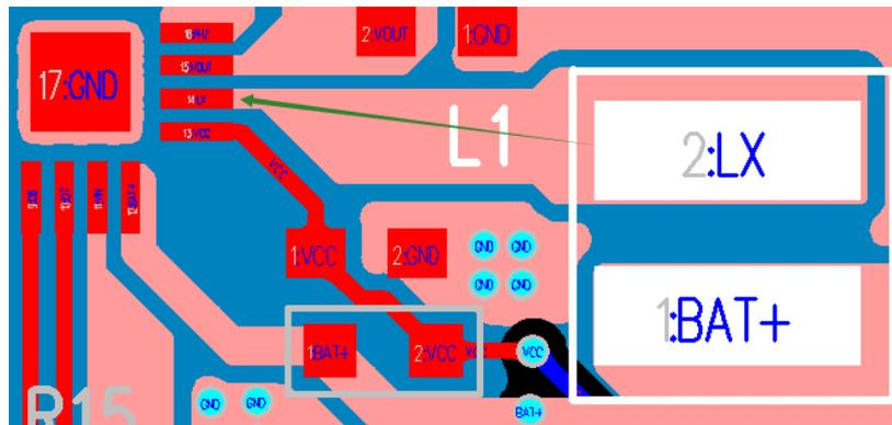
6. It is forbidden to layout any other networks wire under the 5521 chip. Only GND via need to be drilled under the EPAD:
