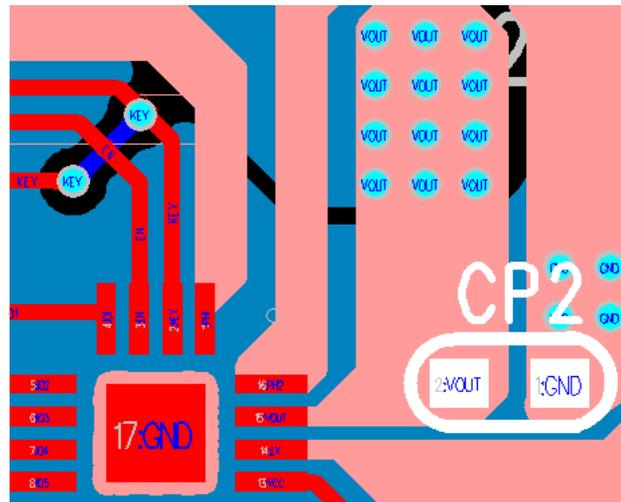
4. BAT pins are shorted together as the positive terminal of the linear charger output connected to the battery. The wiring width needs to be increased to reduce the line resistance to ensure the passage of large current; BAT capacitors should be placed as close to the chip as possible:
