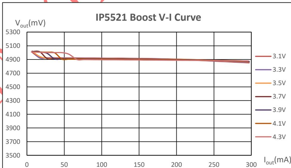
Figure5 IP5521 Boost Output V-I Curve
