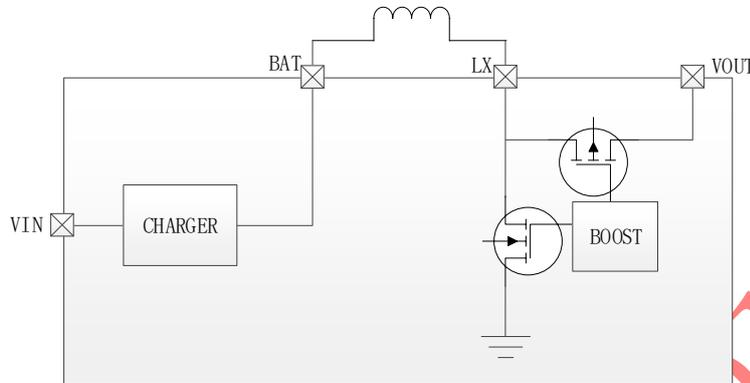
**Figure8 IP5521 Power Path Diagram**
