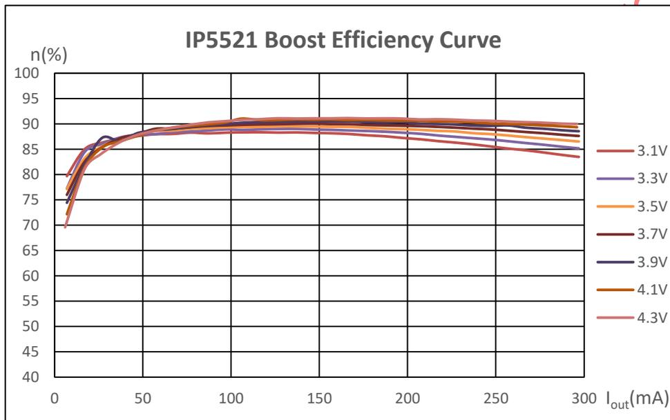
Figure4 IP5521 Boost Efficiency Curve
