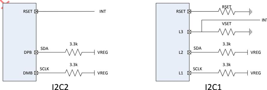
IP5322 support to connect with I2C1 or I2C2 at a time, when I2C circuit is deployed, the two pins will work as I2C\_SDA and I2C\_SCLK and the reused function will be disabled. Under I2C mode, INT signal is high-z at standby and high level at working state, which is used for waking up the MCU.
