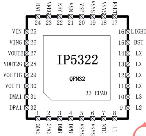
Figure 2 IP5322 Pin Assignments
