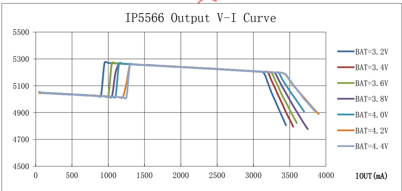
Figure 5 IP5566 Output V-I Curve
