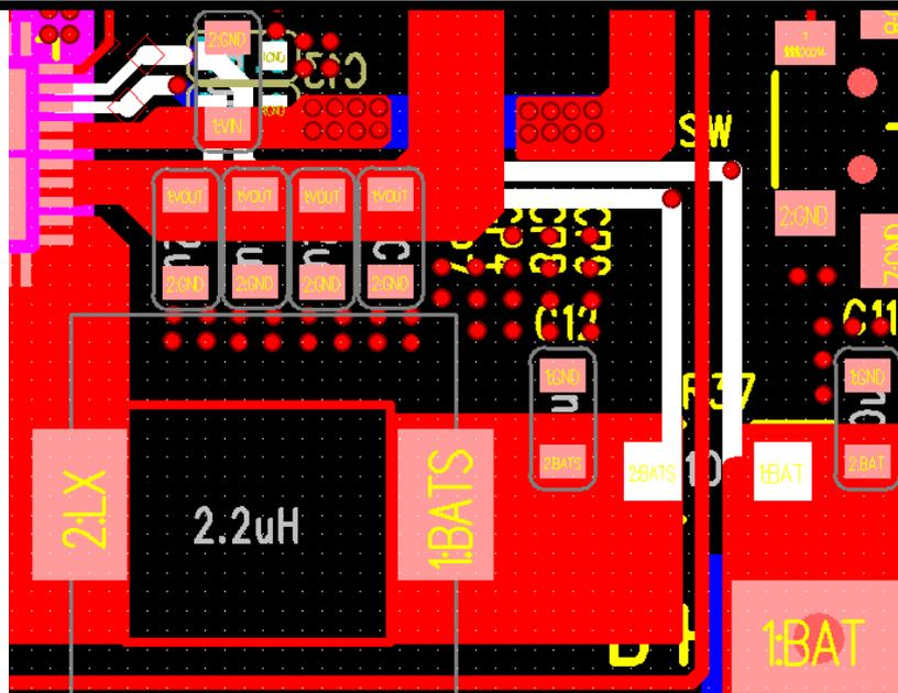
6. The wiring of ADC signals (ADC1, ADCGND, ICOIL, VCOIL) and wireless charging/decode signals (I\_DECODE and V\_DECODE) should be avoided to the wiring of large current (such as VIN, VOUT, etc.), so as to prevent the signal being disturbed and unable to work normally.
